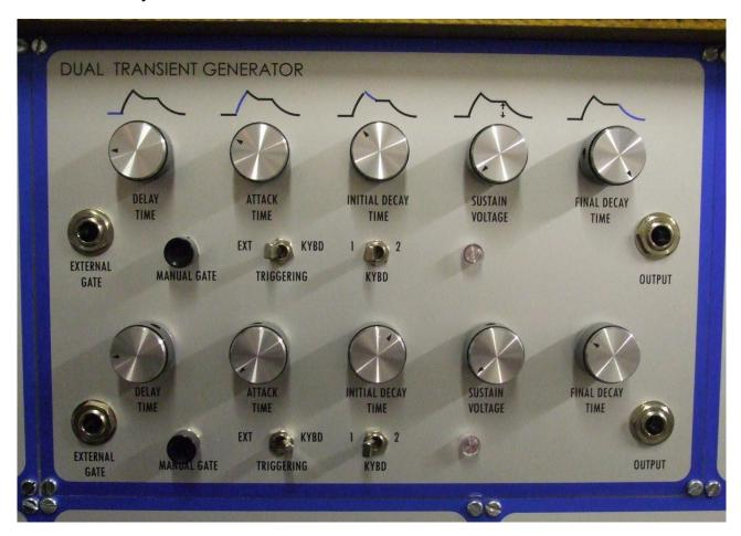
The EA2350 Dual Delayed Transient Generator module contains two independent fourphase electronic music transient generators in a single module. It is based on two EA1350 submodules. With the triggering switch in the external position, the module will produce a four-phase transient when triggered by an external gate:
