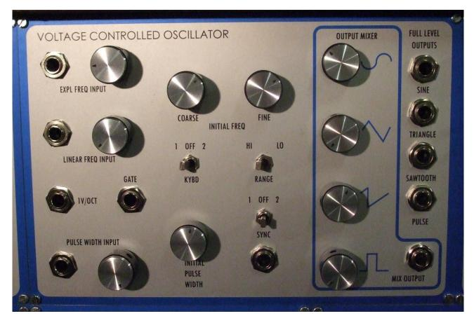
The EA2200 Voltage Controlled Oscillator is a complete, four waveform, exponentially and linearly controlled oscillator with an output mixer. It is exceptionally stable and accurate for use with full size synthesizer keyboards. It contains an EA1201 VCO submodule, and an EA1210 wave converter submodule.
