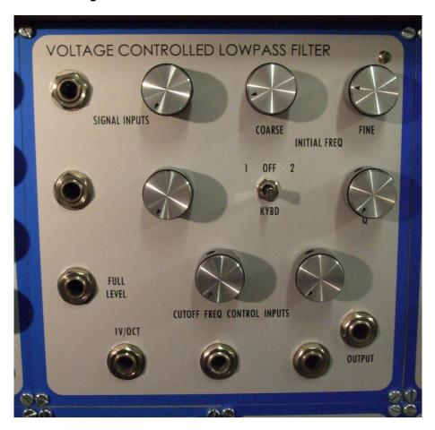
The EA2100 Voltage Controlled Lowpass Filter is an exponentially controlled lowpass filter with variable Q for electronic music applications. It contains an EA1100 VCF submodule.
