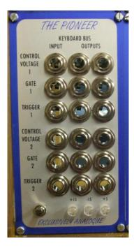
The EA2905 Power Supply Modules are complete power systems for the Pioneer Modular synthesizer. The 2905's front panel contains the power switch and 3 pilot lamp, plus multiple input/outputs for two keyboards. When a keyboard is not connected, the associated system busses can be used for routing any signal by applying via these power supply panel jacks.
