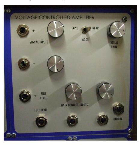
The EA2000 Voltage Controlled Amplifier is an exponentially and/or linearly controlled amplifier for envelope shaping or control functions. It contains an EA1001 VCA submodule.
