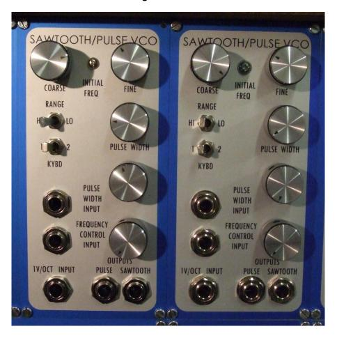
The EA2210 Sawtooth/Pulse VCO is a two waveform exponentially voltage controlled oscillator with many of the features of our 2200 VCO. It contains the stable and accurate EA1201 VCO submodule.
